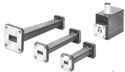
Fig. 8. External mixer connects Spectrum Analyzer to waveguide systems. Two mixers are available, one for X band and one for P, Q and R bands. Taper sections match various waveguide sizes to ridged waveguide of mixer.
